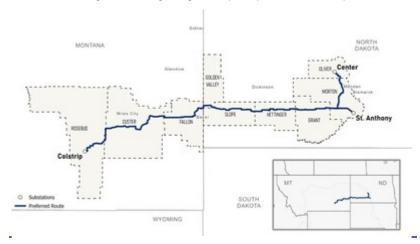
The North Plains Connector will be the nation's first HVDC transmission connection among three regional U.S. electric energy markets the Midcontinent Independent System Operator, the Western Interconnection and the Southwest Power Pool - providing additional flexibility and the sharing of resources across multiple time zones.
